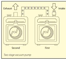
Most refrigeration/air conditioning service technicians use a two-stage high-vacuum pump for the bulk of their service jobs as they can achieve a lower vacuum in less time. The exhaust of the first pumping stage is discharged into the intake of the second pumping stage, rather than to atmospheric pressure.
