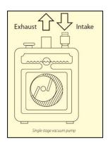
Single stage high vacuum pumps are smaller, lighter in weight and less expensive than two-stage pumps of equal capacity in L/min.
