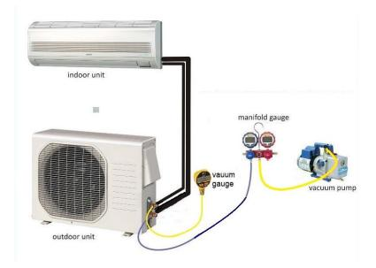
When reading the vacuum created in a refrigeration or air conditioning system, isolate the vacuum pump using an isolation valve and allow the pressure in the system time to stablise before taking a final reading.
